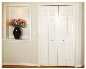
The Bifold range of folding door hardware offers a stable, silent and smooth-opening folding system for cupboard and wardrobe doors that can complement any room. Designed for wooden and wood framed doors, the Bifold system can support a maximum door weight of 14kg and door thickness of between 18-35mm. A range of kits are available to cater for a maximum opening width of 2134mm. A fittings kit is available for when an additional door is required.
